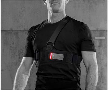
For instance, StrongArm Technologies, has developed the FUSE Platform which includes a wearable device with a variety of sensors, including motion, and an software system which allows for the direct, accurate, and verifiable consideration of the human factors in assessing the safety conditions of the worker. These technologies that include risk management sensors reduce reliability errors to less than a 5% margin of error.<sup>67</sup>
